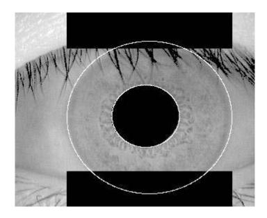
This is the process to remove the extra part of the image. Iris can be divided in to two circles one is iris boundary and second is pupil boundary. For iris localization we use the Dugman's algorithm [1].
