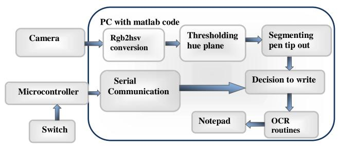
Fig.1: Block diagram of Microcontroller for OCR
