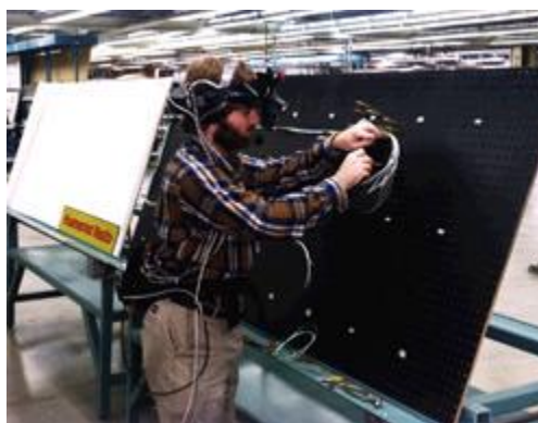
FIGURE 7: Adam Janin demonstrates Boeing's prototype wire bundle assembly application. (Courtesy David Mizell, Boeing)
